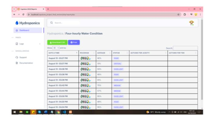
The interface displays a data table presenting water condition metrics like acidity, total dissolved solids, water flow, water level, and temperature and total dissolved solids (TDS), with interactive features for actions and navigation controls for easy browsing.
