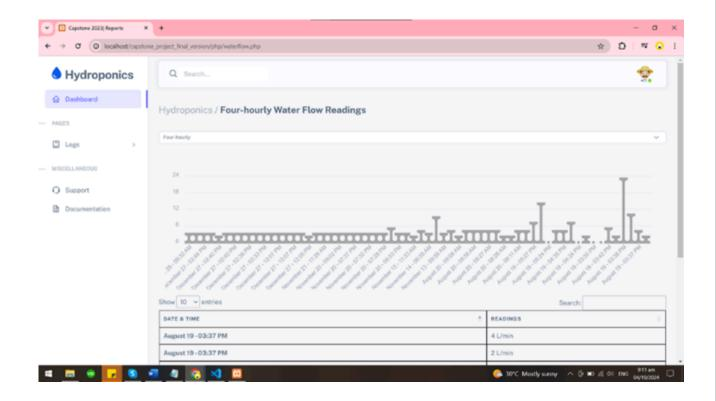
The interface shows the date and time in order, along with water flow measurements in liters per minute. Simple navigation buttons and extra information make it easy to use and understand.
