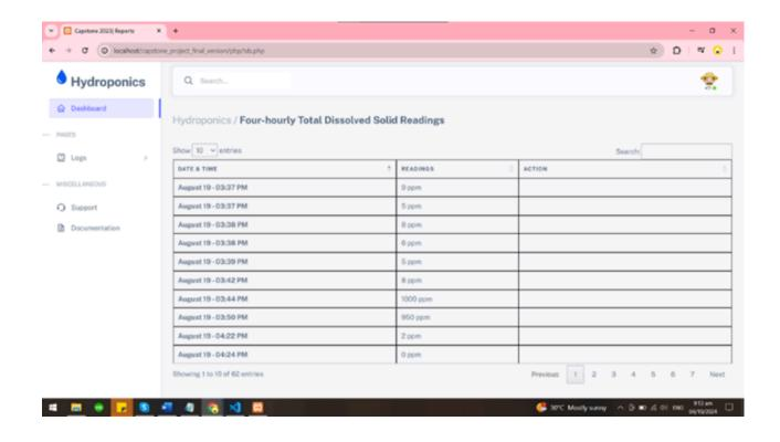
The interface displays a table that shows detailed information on Total Dissolved Solids (TDS), including exact dates and times, actions taken, and extra details. This setup gives a complete view of the data. The logs are organized chronologically and include interactive features for more in-depth analysis.
