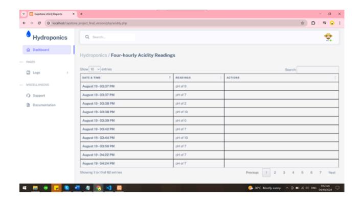
The interface displays pH (acidity) readings in a clear table format. It has columns for date and time, the readings, and any actions taken. The main goal is to show acidity levels recorded at different times, giving a complete picture of the data.
