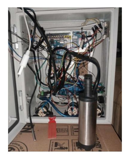
Inside of the Device: A compact array of high-tech sensors arranged to monitor water quality, including indicators for acidity, temperature, dissolved solids, flow rate, and water level.
